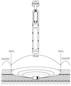
Start by following the suspected path of the pipe and use the **8873** Locator to locate the Sonde. Stop locating when the PEAK reading is found. Then rotate the Receiver as shown in the figure below. When pivoting the Receiver, do not change the vertical position. The Receiver will indicate a PEAK when the Receiver antenna is in line with the Sonde.
