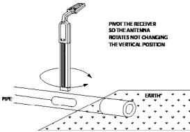
Now move the Receiver side to side (across the path of the pipe) as shown below. When the PEAK if found, the Receiver is directly over the Sonde. Mark this location. Next, check for ghost signals in front of and in back of the Sonde to confirm the location.
