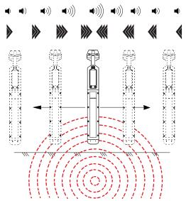
Trace the path by walking away from the Transmitter at a moderate pace. Move the Receiver to the left and right while walking, following the indications.
